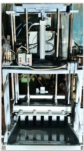
N:B:.The Brick Molding machine's Maximum Mold/ Dice holding capacity/Space is: 800mm \*650mm\* 200mm.
